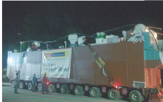
Cutter ladder being loaded on an extendable low loader at fabricator's.
