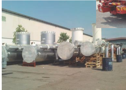
Riser Sections at transit yard awaiting arrival of the conventional ship at Port Klang
