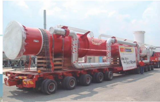
Riser Sections enroute from fabricator to Port Klang on multi-axle hydraulic trailer
